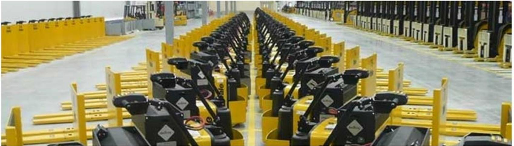
The entire fleet of material handling equipment at the new Walmart Perishable Distribution Centre (PDC) in Balzac Alberta is powered by hydrogen fuel cells.
