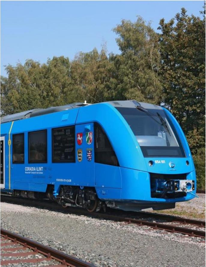
**Brief description:** Hydrails are hydrogen-fuelled regional trains, using compressed hydrogen gas as fuel, to generate electricity via an energy converter (the fuel cell) to power traction motors or auxiliaries. Hydrails are fuelled with hydrogen at the central train depot, like diesel locomotives
